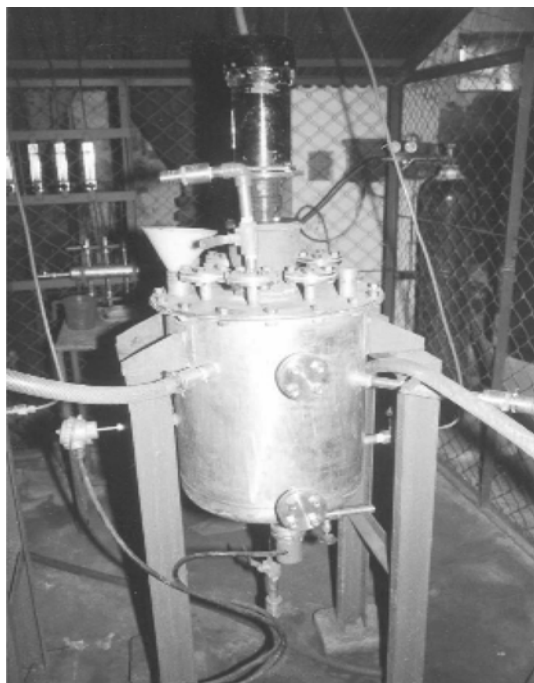
Fig. 1. 40 L capacity bioreactor (Stainless Steel-SS316).
